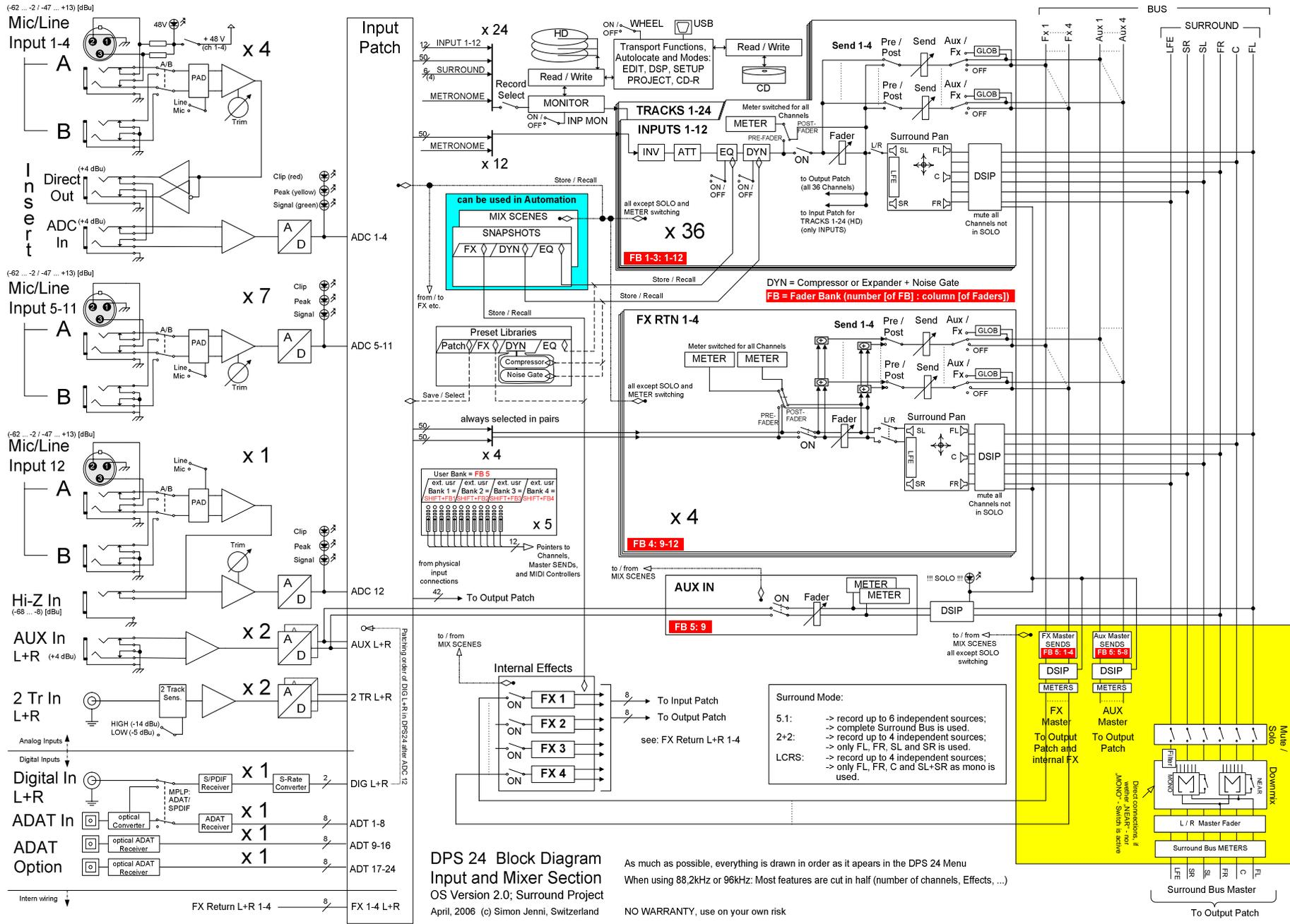
**DPS 24 Block Diagram Input and Mixer Section**
