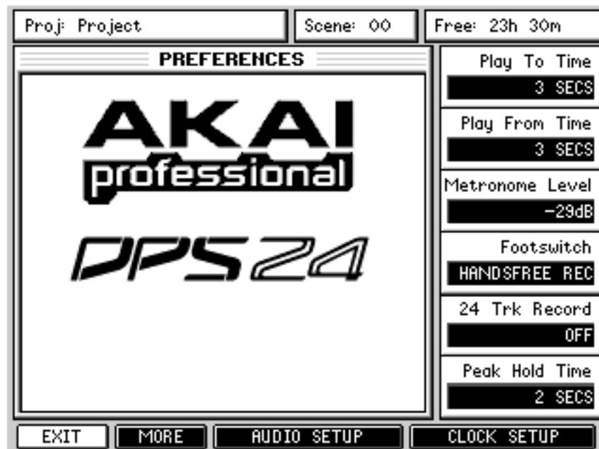
The range is OFF - 1 SEC - 2 SECS - 5 SECS - 10 SECS - 20 SECS - INFINITY. When INFINITY is selected, the peak hold indicator stays on permanently. The setting made here also affects the meter display in ak.Sys TrackView.
