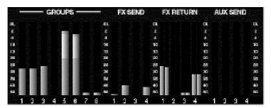
The meters use standard peak meter ballistics which have an instant attack and a decay time of 20dB.second.
